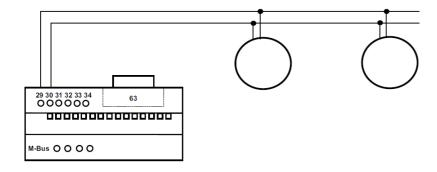
Any cable type may be used as long as the cable is suitable for 36 V / 500 mA. Shielding is not necessary and not recommended since the capacity of the cable should be minimized.
